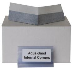
**Aqua-Band** is a wet area grade Elastic Joint Band designed for use in waterproofing wall/floor junctions of internal and external wet areas. Performs as the waterproofing system bond breaker, avoiding the use of sealant beads and backing rod bond breaker methods. Also suitable for sealing movement joints and small expansion joint areas. Consisting of the central rubber section with a flexible polyester fleece making suitable for use with liquid membranes.
