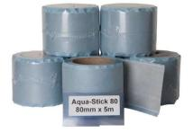
A peel and stick waterproof membrane that is self-adhering, butyl rubber sheet with a polypropylene fleece backing, It has excellent crack bridging capabilities and is suitable to use as a crack suppression membrane underneath tile or stone. Eco-friendly and no odour. Can be tiled on immediately.
